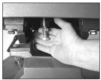
Figure 22. Location of guide pin height lock.
